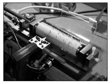
Figure 6. A pneumatic "headless pinner" is used to install steel pins in the roller. As the blank roller is rotated, a lead screw advances the roller and mounting stage along a slide rail. This creates the one-tenth of an inch per revolution spiral path required for the pins.
