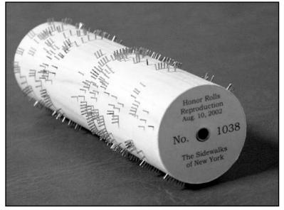
Figure 11. A reproduction of an original roller, #1038 *The Sidewalks of New York*. A reader attachment on the pinner allows originals to be read into the computer. The roller is clearly labeled as a reproduction.
