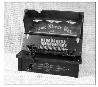
Figure 2. The "Home Music Box" is the basic vacuum-operated model of the Gem Roller Organ with a front cover and name board added for "show." Here the front cover is shown open revealing the double row of valves.
