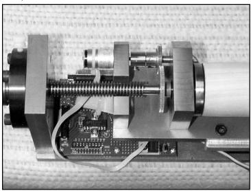
Figure 7. A small stepper motor mounted on the roller stage is geared to the roller and the lead screw. The nut for the lead screw is adjustable to precisely locate the spiral path for the pins.
