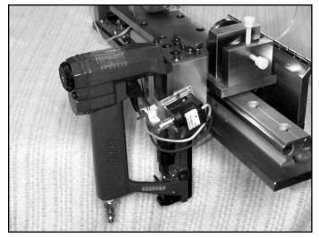
Figure 8. The headless pinner can be fired automatically with a solenoid or triggered manually.
