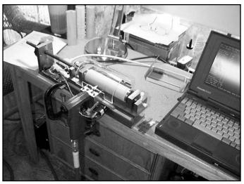
Figure 10. A laptop computer controls the automatic pinner over a standard parallel port.
