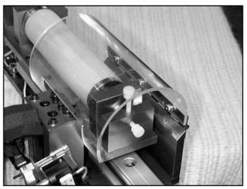
Figure 9 A shield protects the operator from the unlikely possibility of an errant pin.
