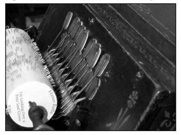
Figure 3. The pins on the roller lift the valves to play the 20-note scale. The roller plays for about 40 seconds in three revolutions and then returns to the beginning.
